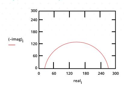
The Nyquist Plot for a Simplified Randles cell is always a semicircle. The solution resistance can found by reading the real axis value at the high frequency intercept. This is the intercept near the origin of the plot. Remember this plot was generated assuming that  $R_s = 20 \Omega$  and  $R_p = 250 \Omega$
