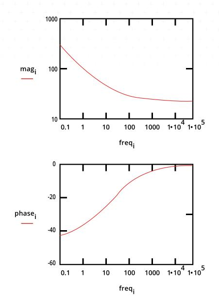
Adding a double layer capacitance and a charge transfer impedance, we get the equivalent circuit in Figure 19. This is the Randles Cell; the name is taken from an article by J.E.B. Randles in the Discussions of the Faraday Society in 1947. Since there is no simple element to model a Warburg impedance, it isn't possible to construct a dummy cell that models the Randles Cell.
