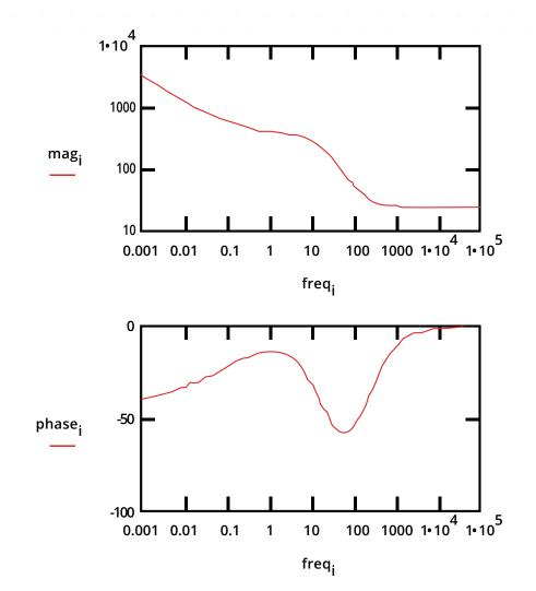
Figure 21. Bode Plot for the Mixed Control Circuit
