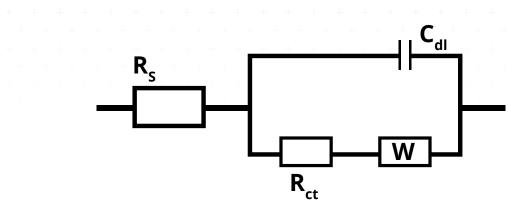
This circuit models a cell where polarization is due to a combination of kinetic and diffusion processes. The Nyquist Plot for this circuit is shown in Figure 20. As in the above example, the Warburg coefficient ,  $\sigma$ , is assumed to be about 150. Other assumptions:  $R_s = 20 \Omega R_{ct} = 250 \Omega$  and  $C_{dl} = 40 \mu$ F.
