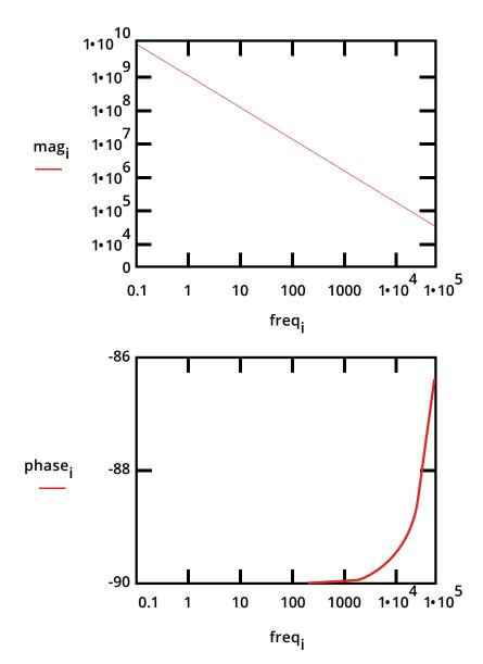
Water uptake into the film is usually a fairly slow process. It can be measured by taking EIS spectra at set time intervals. An increase in the film capacitance can be attributed to water uptake.
